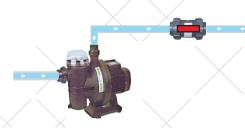
The water circulates normally, when the valve is open and the pump is running.
